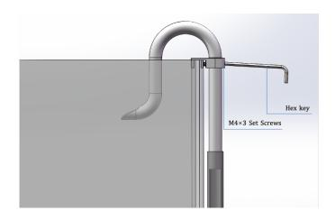
\*The METAL PIPE FLOW for Inflow has an end cap on the inflow strainer. By removing the end cap, cleaning becomes easier.
